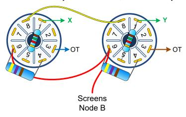
This mod replaces two lug jacks with switching jacks for improved operation. The instrument jacks have been rewired as typical Fender style high/low jacks. A grid stopper resistor has been added at the tube socket for the Mic channel.
